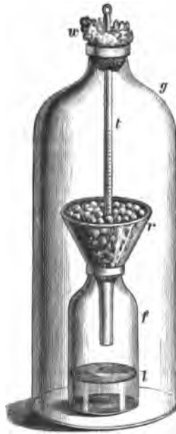
FIG. 37 (from Prantl, after Sachs). The moist seeds are placed in the funnel r , which is placed in the neck of the bottle f containing some solution of caustic potash l to absorb the carbon dioxide evolved. The whole is covered by the bell-jar g , through the neck of which passes the thermometer t : the bulb of the thermometer is covered by the seeds in the funnel. The cotton-wool w which holds the thermometer in the neck of the bell-jar admits air.
